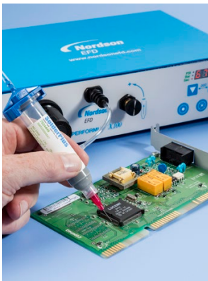
Dispensing SolderPlus® solder paste on PCB boards.
